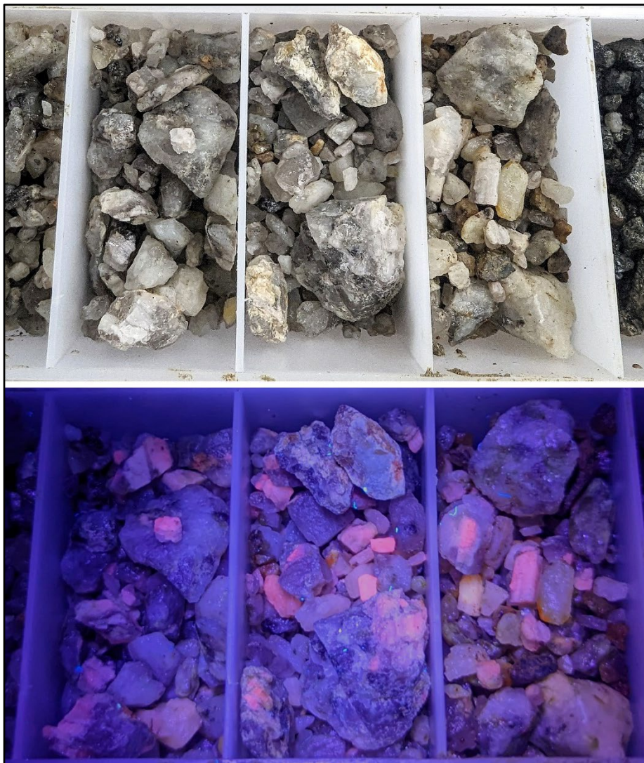
Figure 3: FSIR0010 chip trays from 43 – 46m downhole depth. Natural light (top) vs ultraviolet (UV) light at 365nm (bottom) showing spodumene crystals glowing pink under UV light.
