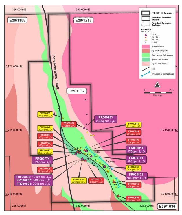
Figure 2: The Breakaway Dam project area (E29/1037) including all mapped pegmatite, granite and quartz vein locations from recent field trips. All samples >200ppm Li₂O are highlighted. The geological base map is courtesy of GSWA, the legend includes all geological units within the project area.
