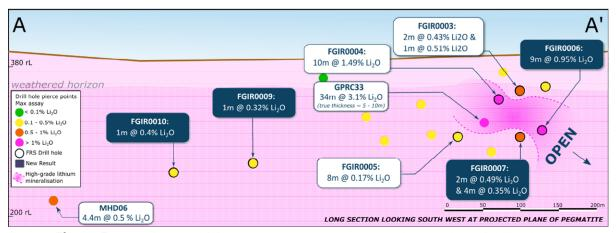
Figure 5: Long Section of Giant pegmatite body showing pierce points of drilled holes
